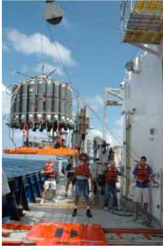
Putting the large CTD in the water, they are collecting phytoplankton samples as well as collecting data on the water column
