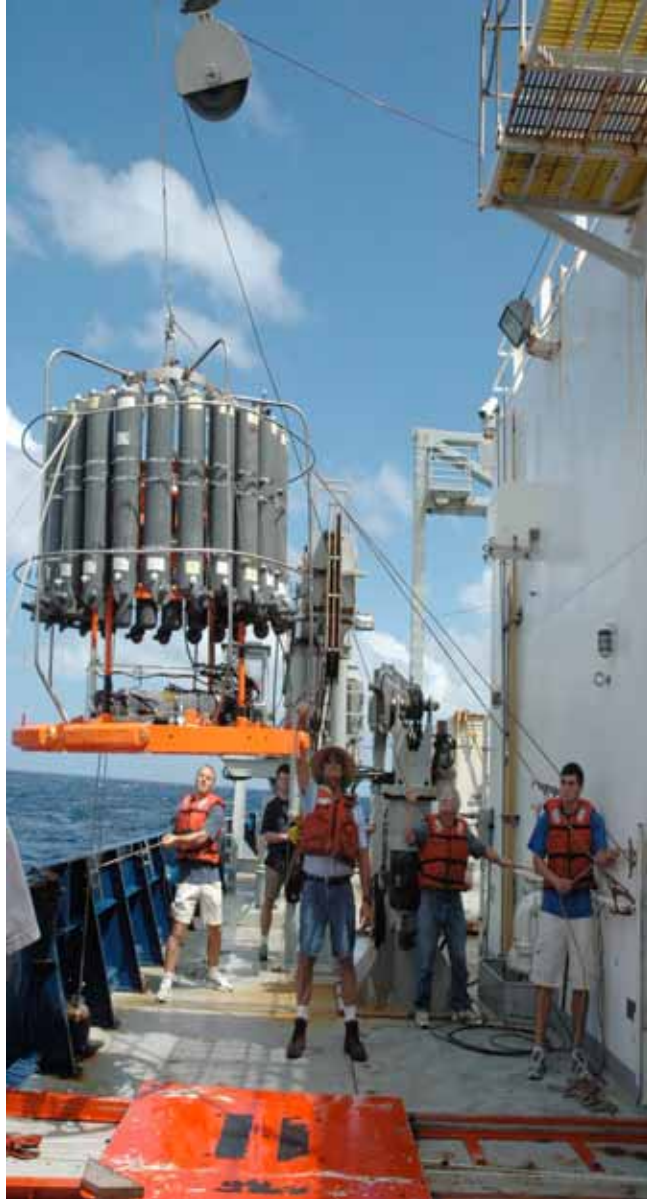
Lift off! Launching the CTD package from the staging bay. 1 st cast of the day.
