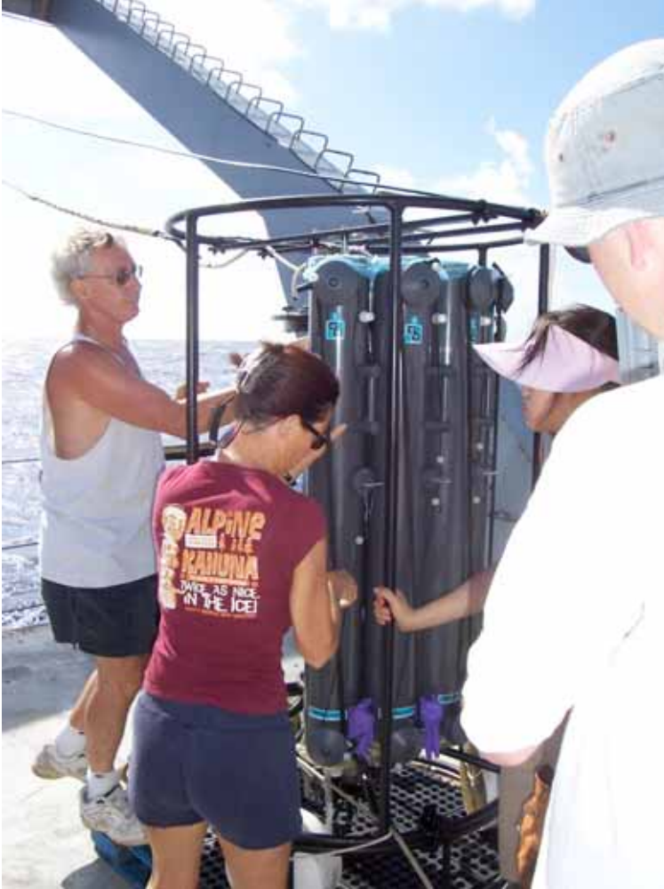
Dr. Measures instructing us how to load the bottles on the CTD rosette.
